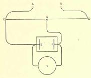
primary batteries, secondary batteries, dynamo or lightning circuit. The electrolytic cell is connected so that one pole E connects with C and the other pole F connects with the movable point or slider G so that any point of the conductor CD can be selected and any voltage from zero (when G is at C) to the full
