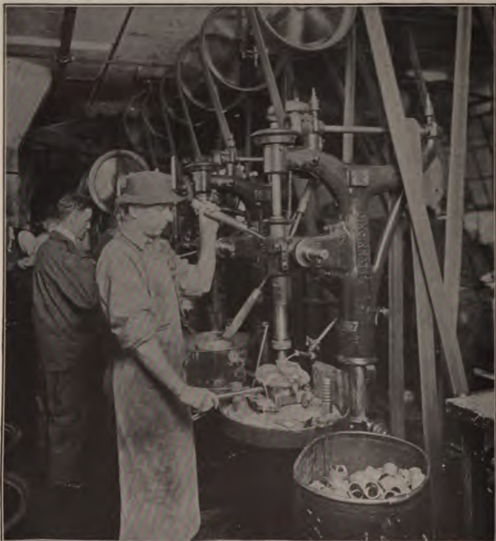
Bushings Job. Line of Drillers for Rough-Boring Bushings Castings. Ford Chuck on Driller Table. See Page 289 for Chuck Construction
