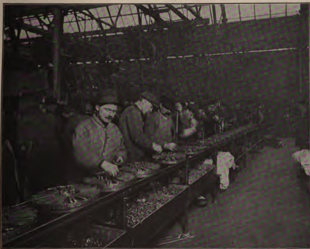
Assembling the Flywheel Magneto. A Characteristic Example of Team Work The work is moving toward the back of the picture, approaching completion by successive operations as it passes from team to team
