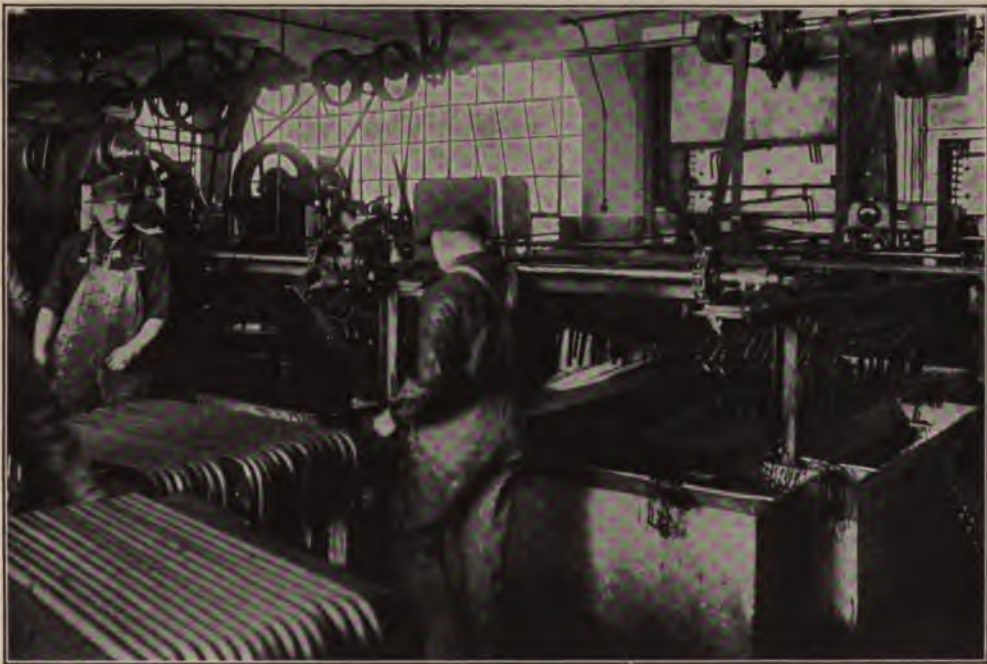
Enameling the Wind-Shield Frames, Showing Dipping Tanks and Draining Conveyer
