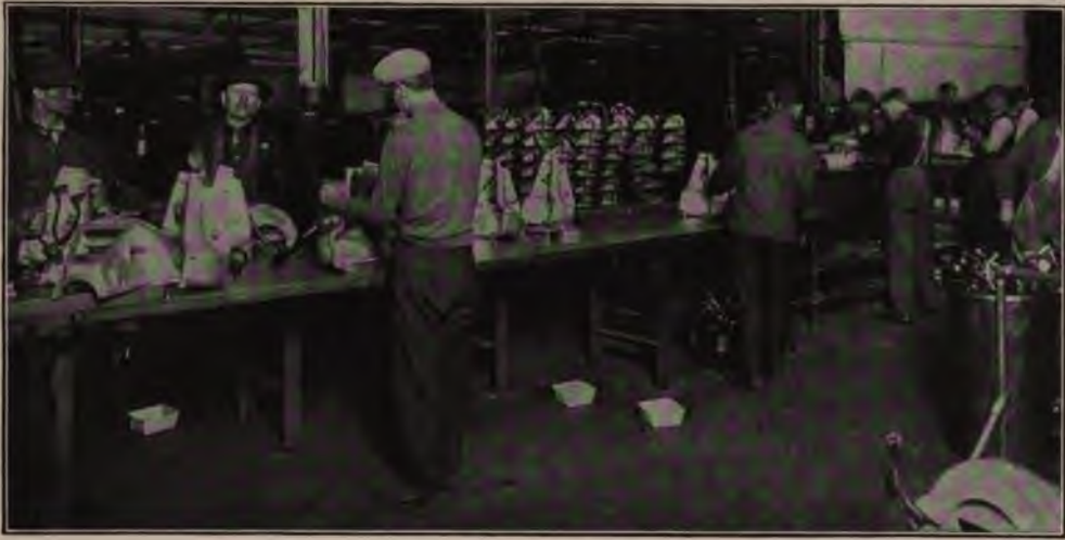
Assembling Transmission Casings
