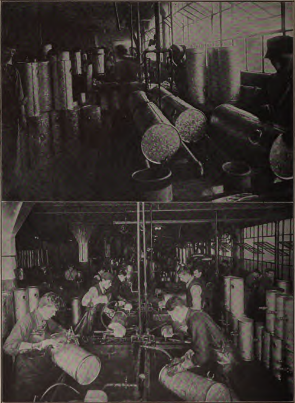
Above: Soldering Longitudinal Seam of Gasoline Tank. Below: Testing Tanks with Compressed Air under Water
