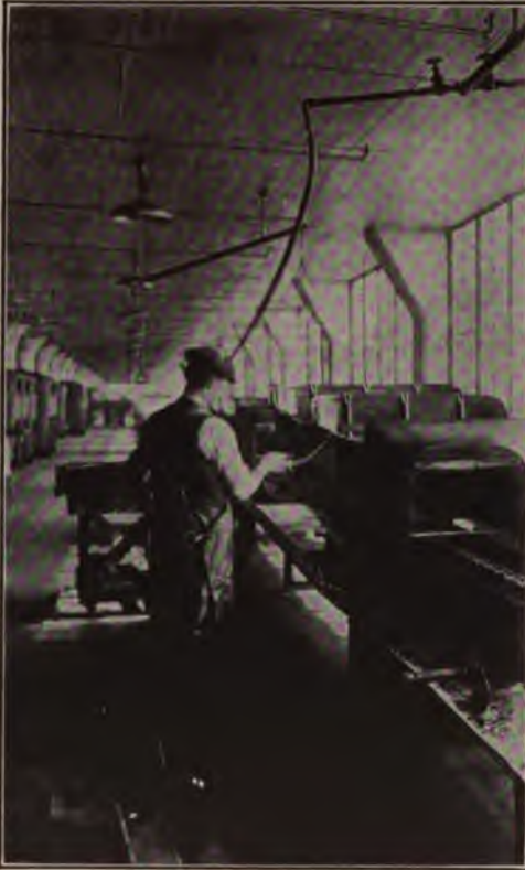
Flowing on the Second Coat of Blue Black Note type of nozzle used, and drain tanks in each side of track
