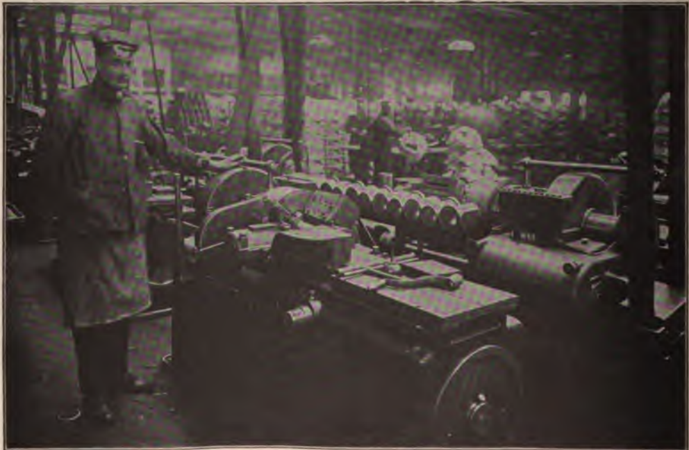
Rough-Turn and Cut Off Piston Ring on Potter & Johnston Special Automatic Machine
