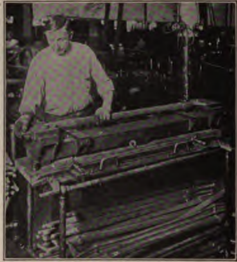
Inspecting Rough Axle Bodies T-202, Coming from the Heat-Treating Department
