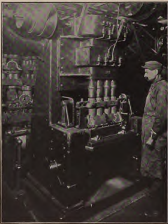
Operation 8 on Cylinder Casting. Finish-Ream Four Cylinder Bores at Once Foote-Burt machine
