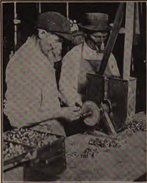
Operation No. 3. On T-4446 Smoothing and burring on Ford machine and Ford rotary files
