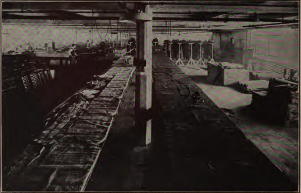
Cutting Out Material for Cushions and Backs Note electric knife used on right-hand table
