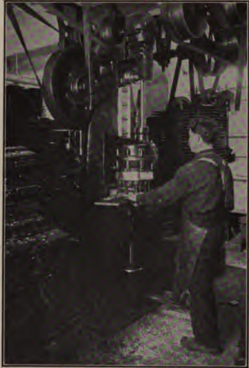
Spindle Punch - Drilling Machine for Making Wood-Screw Holes in Floor Boards
