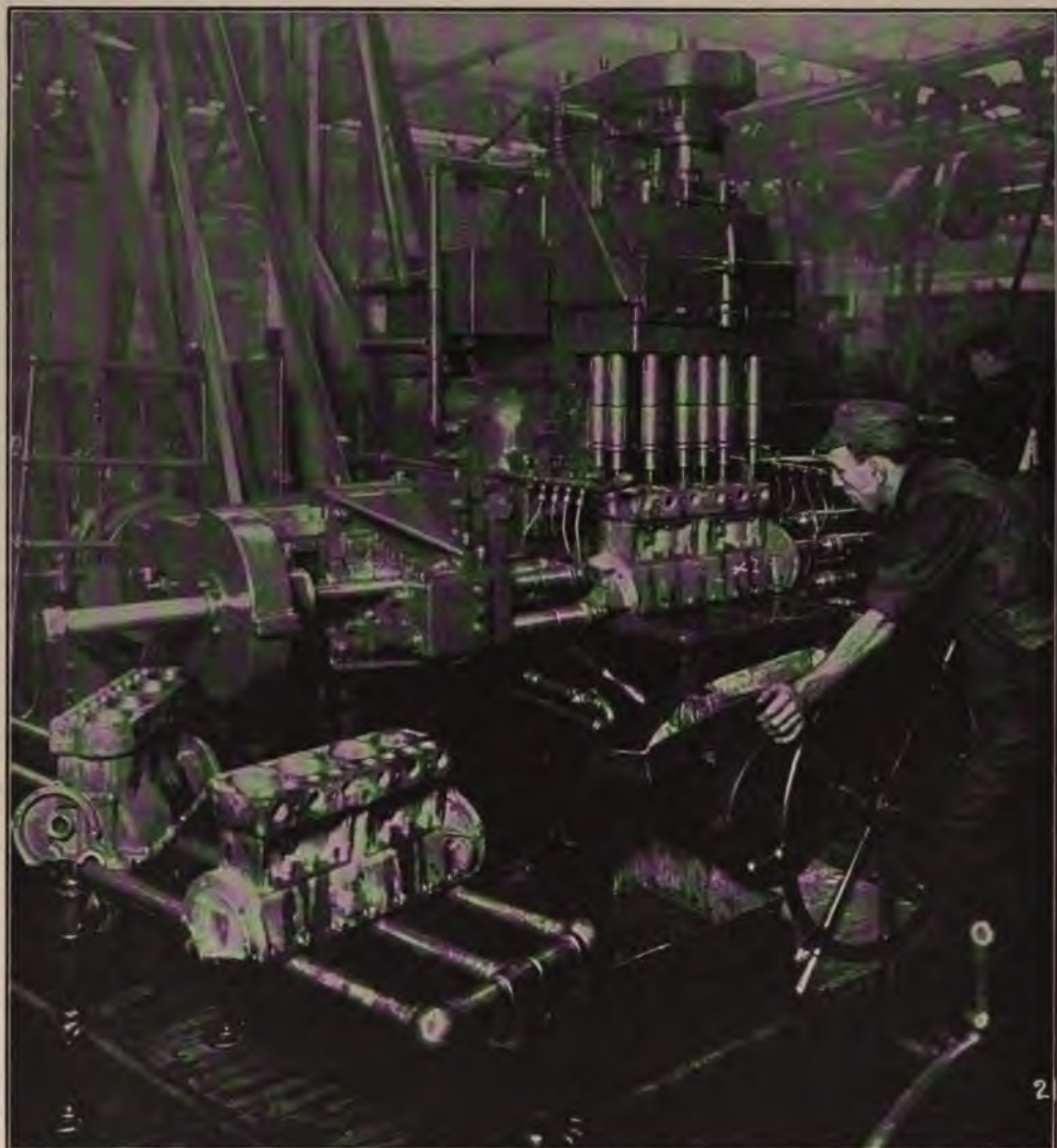
Operation 28 of Cylinder-Finishing Series. Tap 24 Holes from Three Directions Last machining operation. All subsequent operations go in the motor-assembling series, fully described in Chapter IV. Note steel-pipe work-supporting ways, lower left corner. Foote-Burt machine
