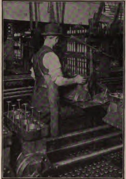
Operation 15—Grinding in the Valves The work of two men was saved by moving this Foote-Burt machine from its original place on the floor into the assembling line.
