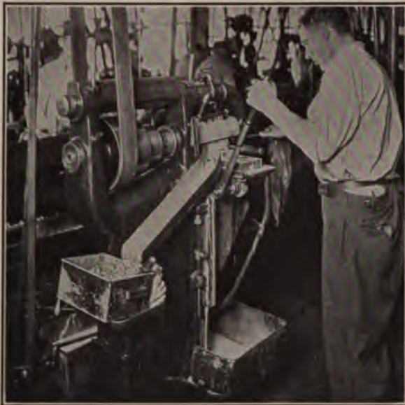
Operation 1 on Commutator Contact Head, T-4462 With a gang mill, cut 10 pieces at once from a crescent-section steel bar
