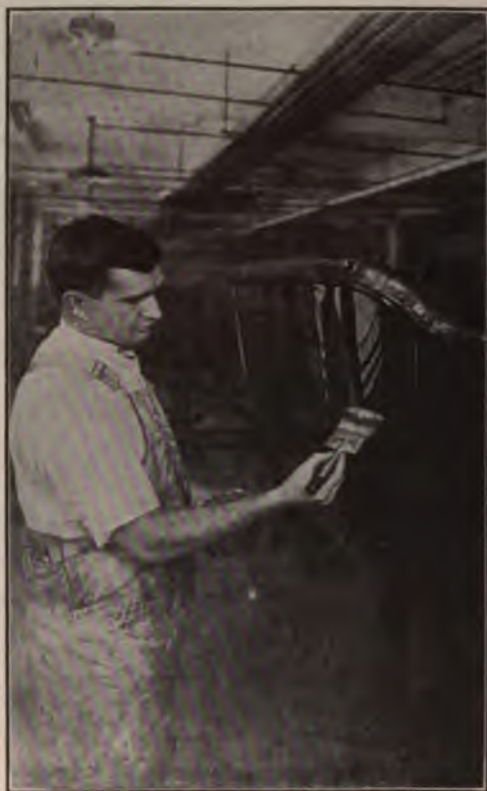
Giving the Body Its Final Touching Up after the Finish Varnish Coat
