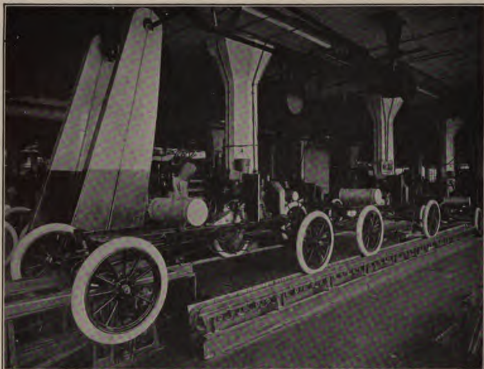
Chassis Leaving Rails on Which the Axles Slide, to Run on Its Own Wheels The sheet-steel casings enclosing the chain-driving belt are shown at upper left. All bolts which could touch workmen in these assembling lines are fully encased
