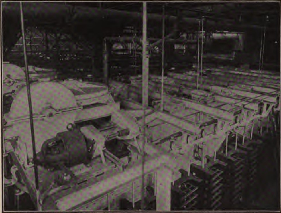
Top View of Double Revolving-Chain Core-Oven
