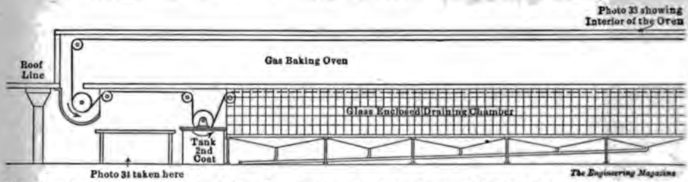
Sectional Diagram of Ford Fender-Enameling System. Half the Length is Shown above. The Section is Completed on the Opposite Page
