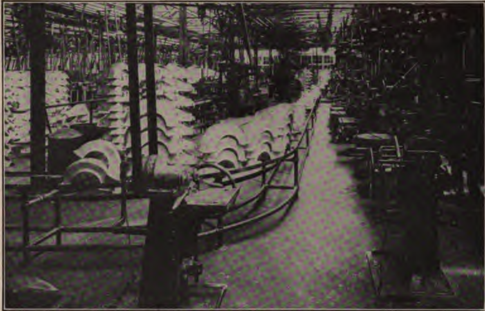
Transmission Cover Slide-Way. Early Construction, Built Up of Steel Tubes and Regular Fittings
