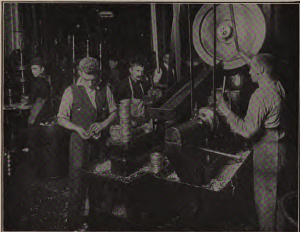
Two Lathes and Power Press for Finishing Large Thrust Washers of Babbitt Metal At left, inspector and two lathe hands. The lathe hands face each other, and the tail-stock ends of the lathes are set close to the power press. The lathe hands take washers as they come down the slides, with outside and inside edges finished, from the press, face the slides and cut a spiral groove in each side, and then drop the finished piece into the short slide marked 4, seen between the lathe men. The washers slide to the end next the inspector, who stacks them on his table for inspection
