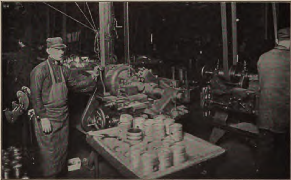
Finish-Turning of Pistons
