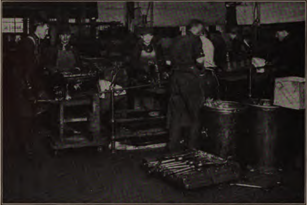
Operation 84—Paint the Motor and Remove it from the End of the Assembly Line to a Small Wooden Stand on Rollers
