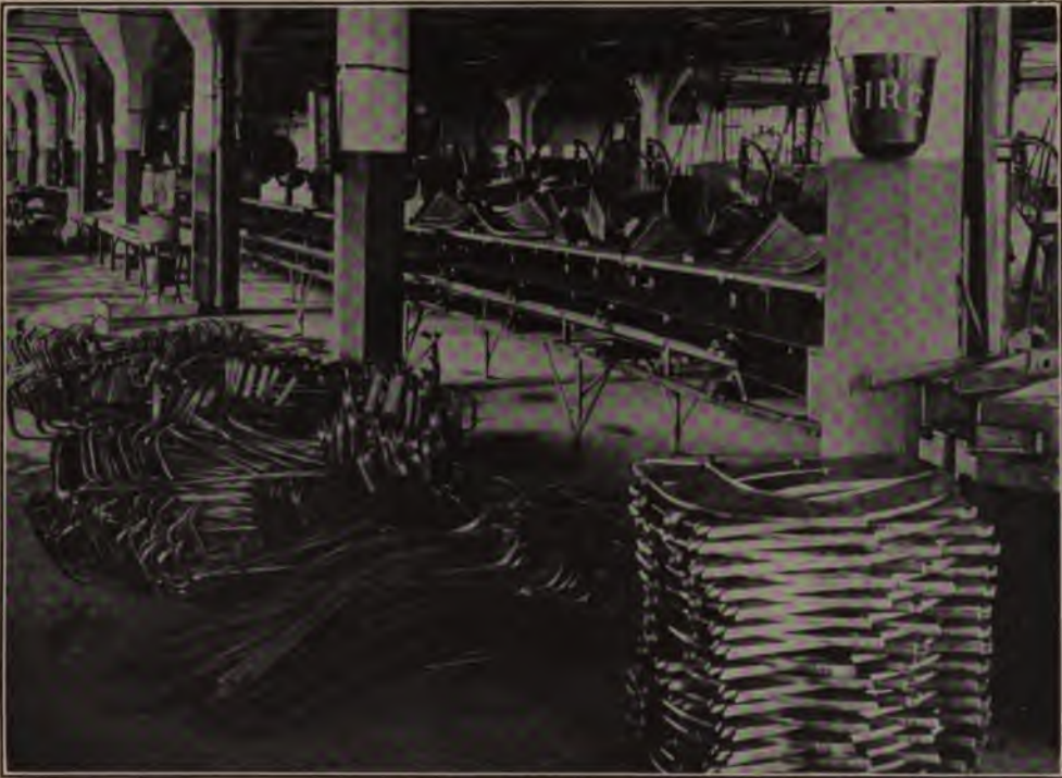
Horizontal Conveyor Belt Used in the Mud-Guard Department to Carry Away Completed Work
