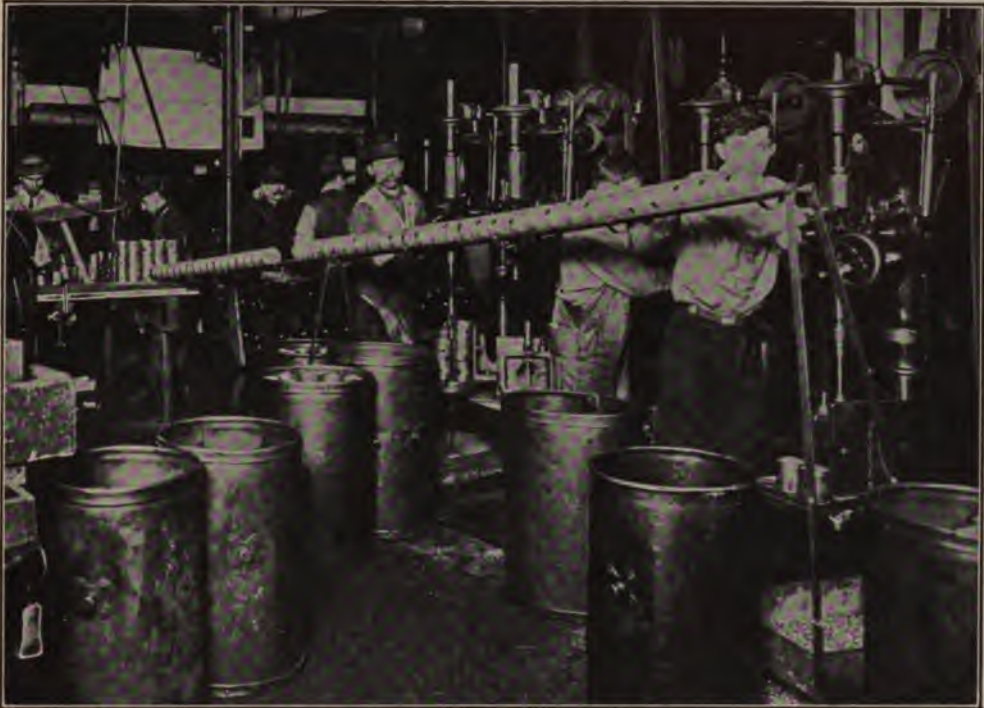
Piston Gravity Slide from Four Drilling Machines to Piston, Pin, and Connecting Rod Assemblers
