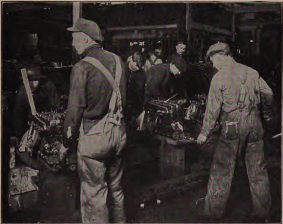
The Man at the Left is Numbering the Motor. The Man at the Right is Trying the Standard Starting Crank for Its Engagement with the Crank Shaft
