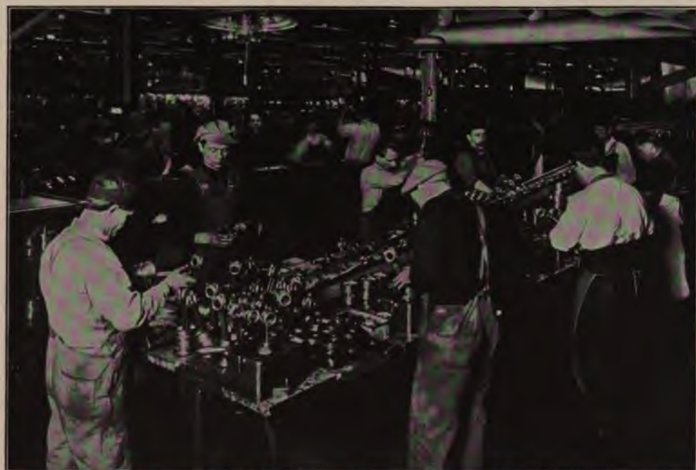
Another View of the North Bench for Piston and Rod Assembling Showing four assembling shelves at the left; the inspector, also at the left, is trying the stiffness of the rod movement
