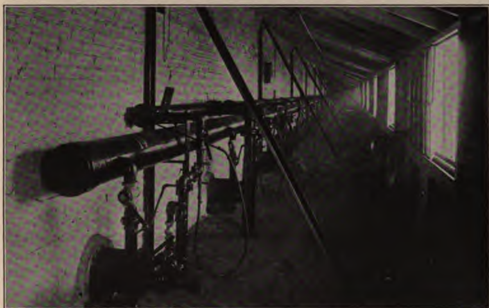
Outside of the Gas-Heated Ovens, Built on the Roof, in Which the Fenders Are Baked
