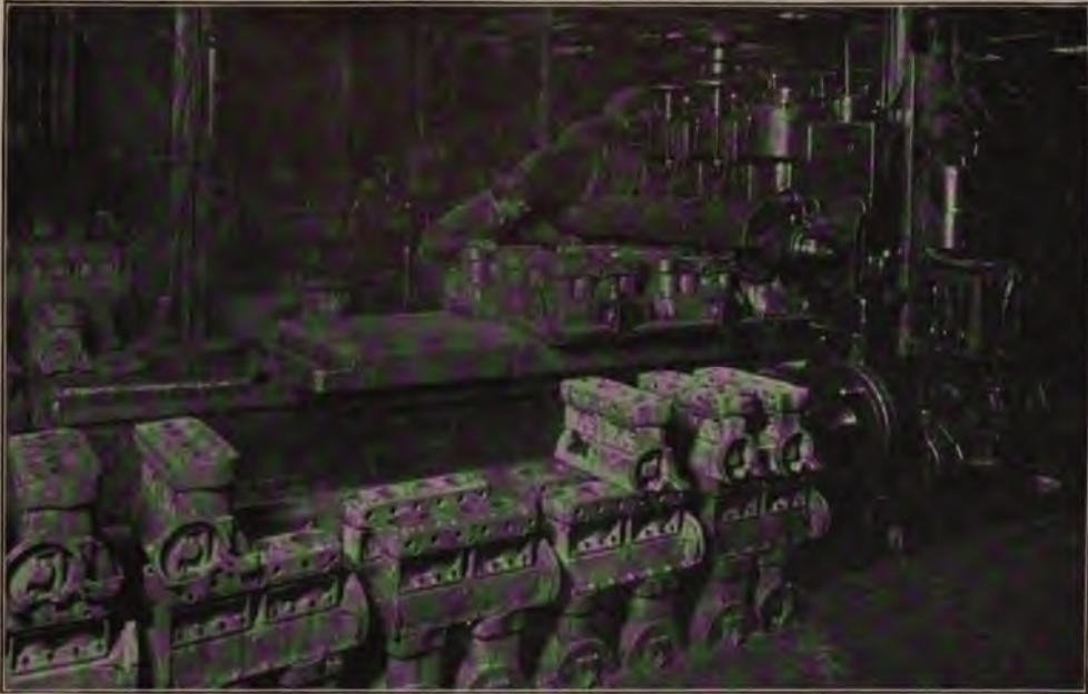
Operation 4 on Cylinder Casting. Surface Tops of Cylinders, and Mill Top-End Sides Ingersoll milling machine
