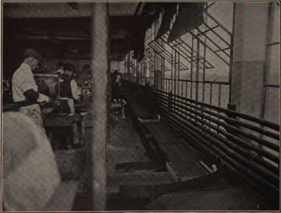
Radiator Job. Three Endless Belts, Two at Right Angles to the One Shown Belt 18 inches wide, speed 33 feet per minute. Saves work of two men with trucks
