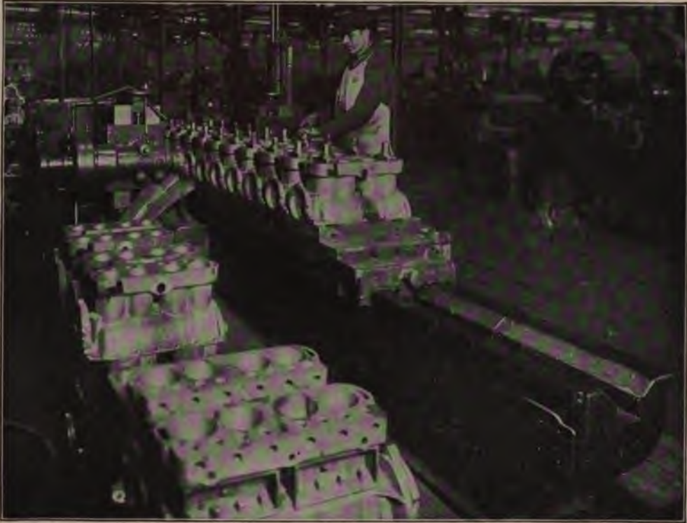
Operation 7 on Cylinder Casting. Milling Both Ends of Cylinders at Same Time Ingersoll two-spindle milling machine
