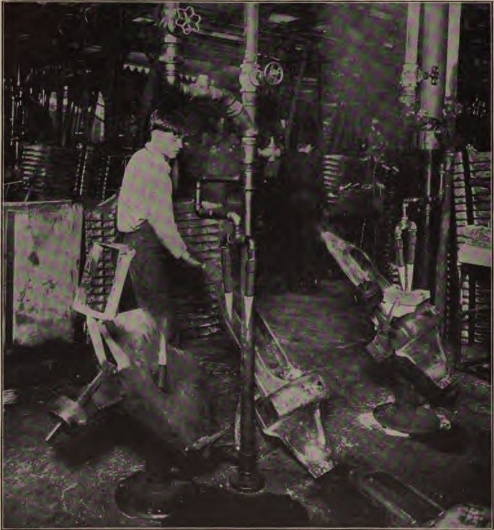
Supplementary Operation 12 on Crank Box. Braze Globe Seat to Crank-Box Shell Stationary flames below, with swinging flames above. Four brazing fires, independent but close together, are used by one man
