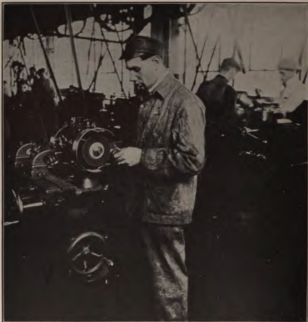
Broach Grinding, Norton Elastic Wheel \frac{1}{16} to \frac{1}{8} inch Thickness, Broach Held in Both Hands
