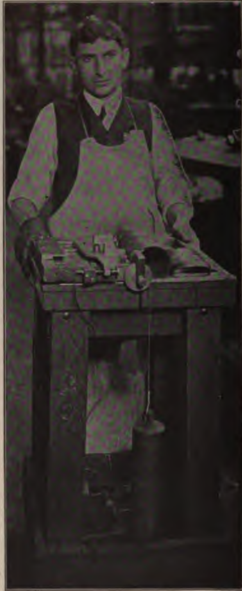
Inspecting Piston Rings for Closing Resistance
