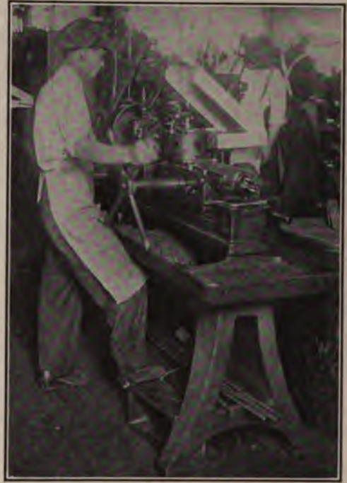
Making the Stud Fiber-Insulation Bush, T-671
