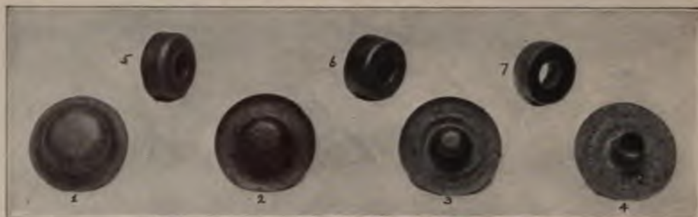
Seven Successive Stages in the Production of the Fan-Belt Pulley
