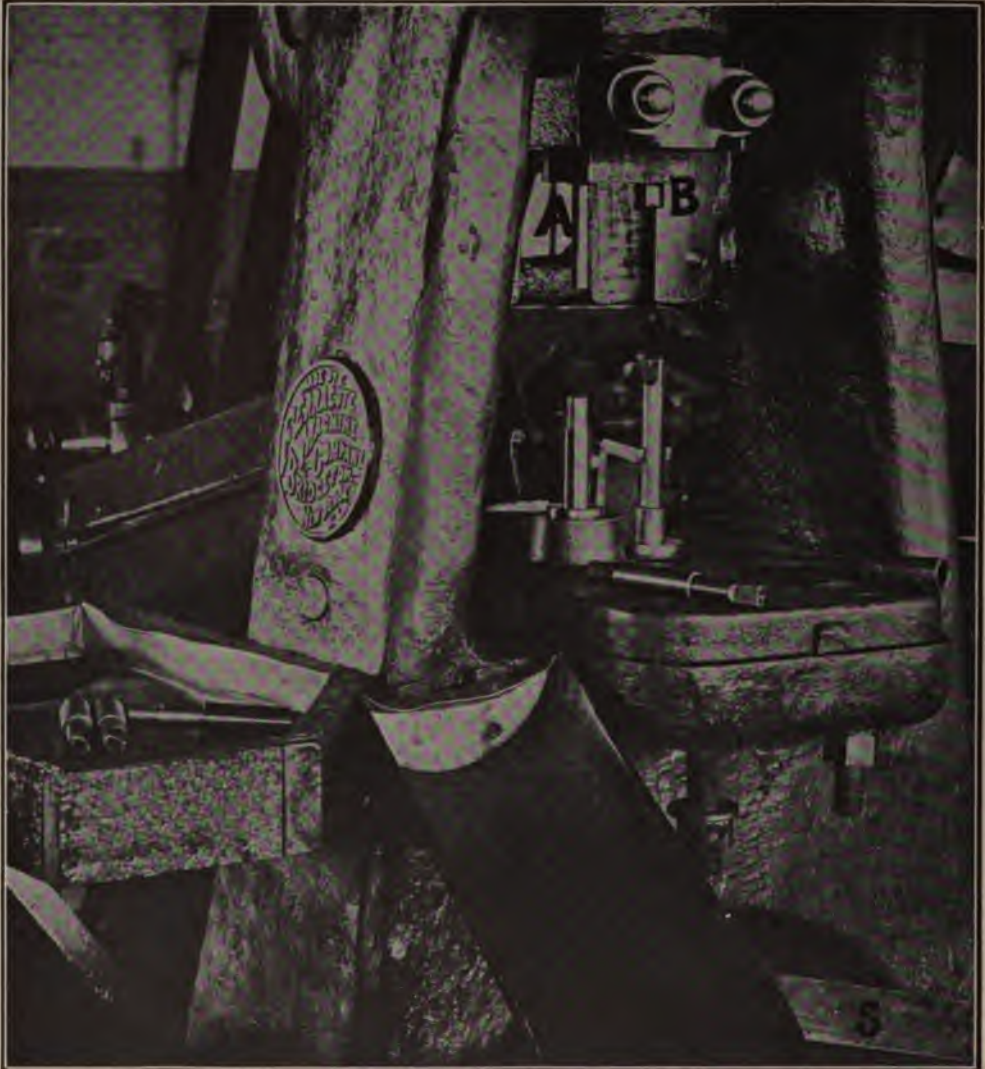
Placing Bushes on Arbors, and Forcing Arbors Out of Bushes; Simultaneous Operations. See also Page 297
