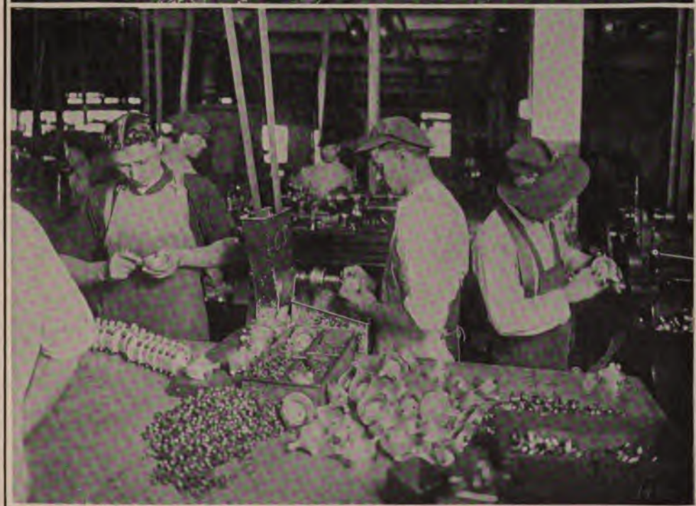
Above, North End of South Bench, Disassembling Outfit. Below, Operation 6, Assembling Contact-Studs and Hex Nuts
