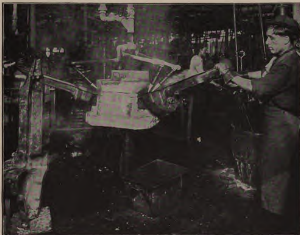
Supplementary Operation 11 on Crank Box. First Braze Braze rear-end annular drop-forging reinforce into rear end of crank-box shell
