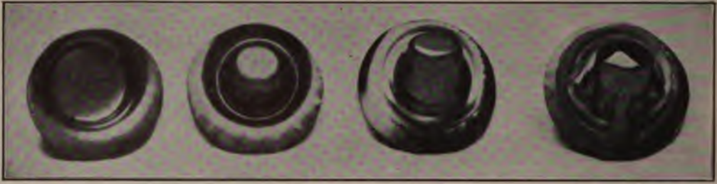
Photograph Showing Successive Changes in Form of Steering Column Flange Note that between picture two and three the metal is turned inside out
