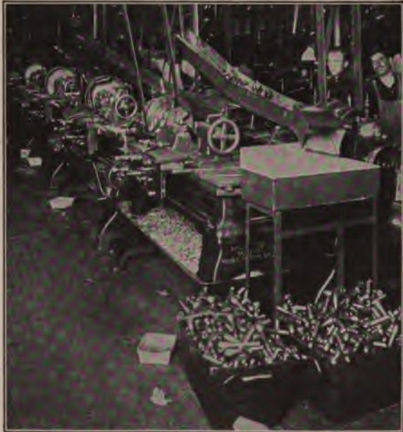
Rough- and Finish-Turn T-203 and T-204 on Reed-Prentice Lathes
