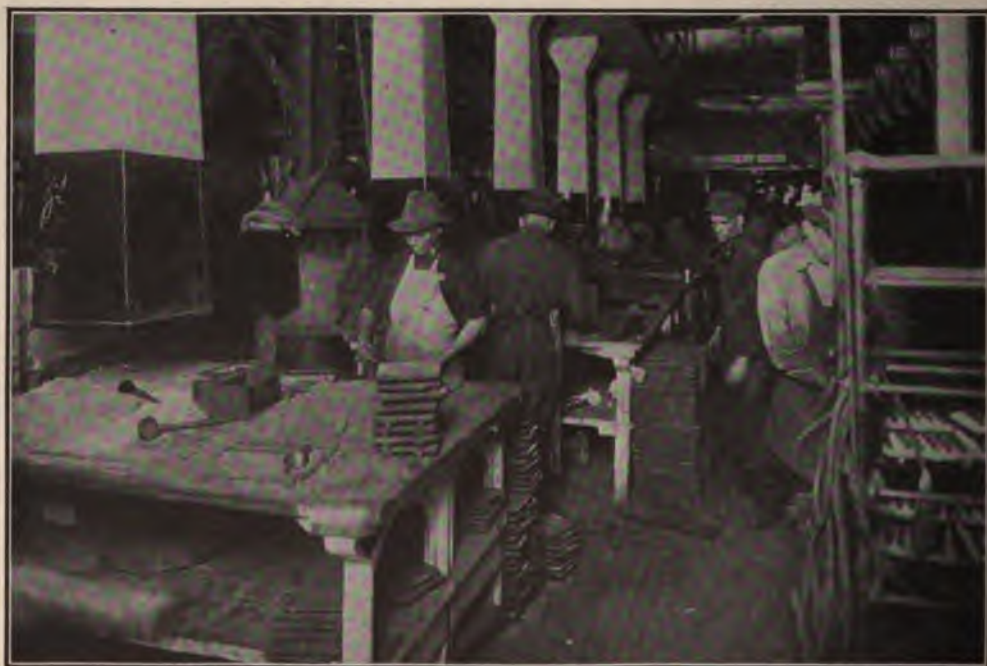
Jobbing Core-Makers at Work under Core-Sand Gallery Core-sand chutes from gallery, seen from the left, along rear of picture. This gallery was devised by the Ford engineers and is believed to be unique
