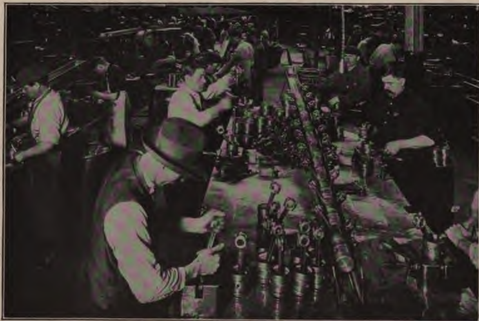
Piston-and-Rod-Assembling Bench with Men at Work South bench, looking east; inspector at left front.
