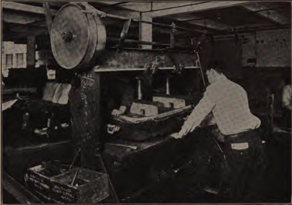
A Cushion Press in the Upholstering Department Here the hair is squeezed down and the buttons are clinched
