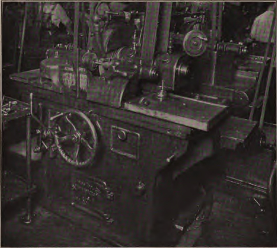
Landis Grinder with Broad-Face Wheel for Grinding Full Length of Cylindrical Parts of Spring Hangers T-91 1/2 and T-246
