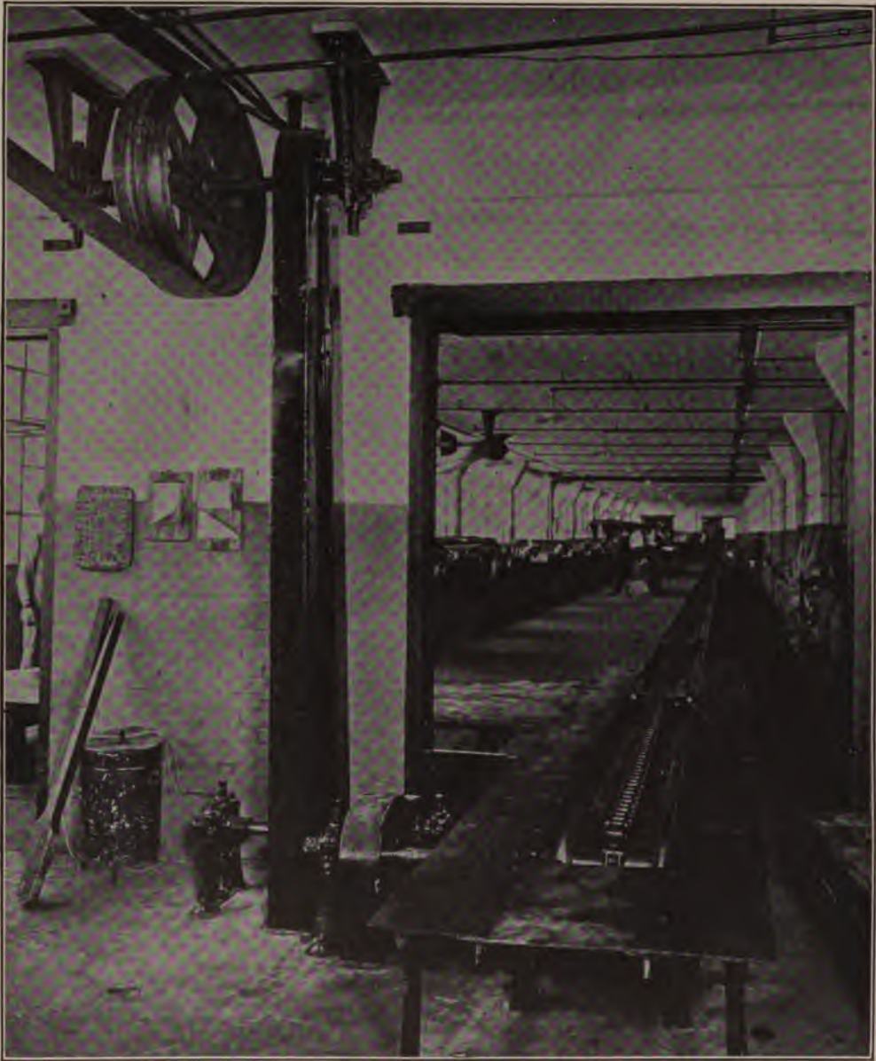
North End of Body-and-Top-Assembling Lines, Showing Drive of the Chains
