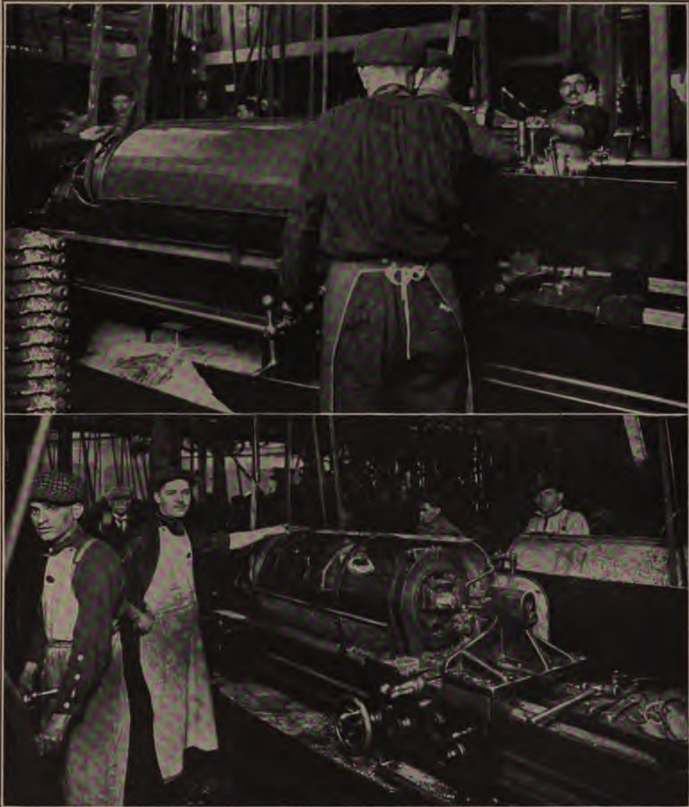
Above: Guard on Lathe Used for Turning End of Crank Case, Shown Closed. Below: Same, Shown Open
