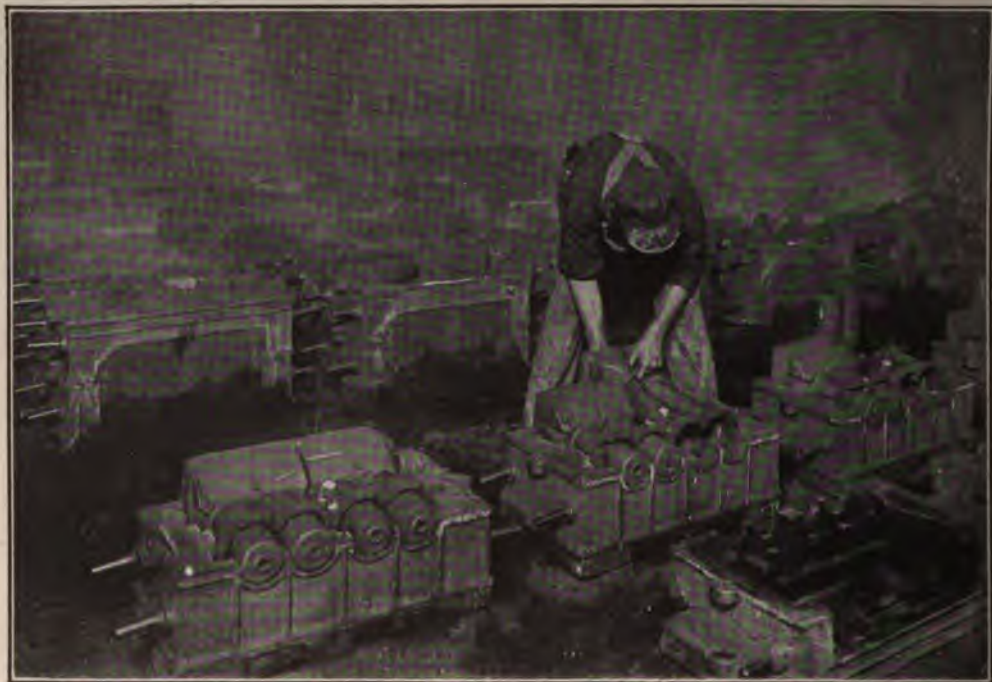
Cylinder Moulding Floor. Setting the Barrel Cores
