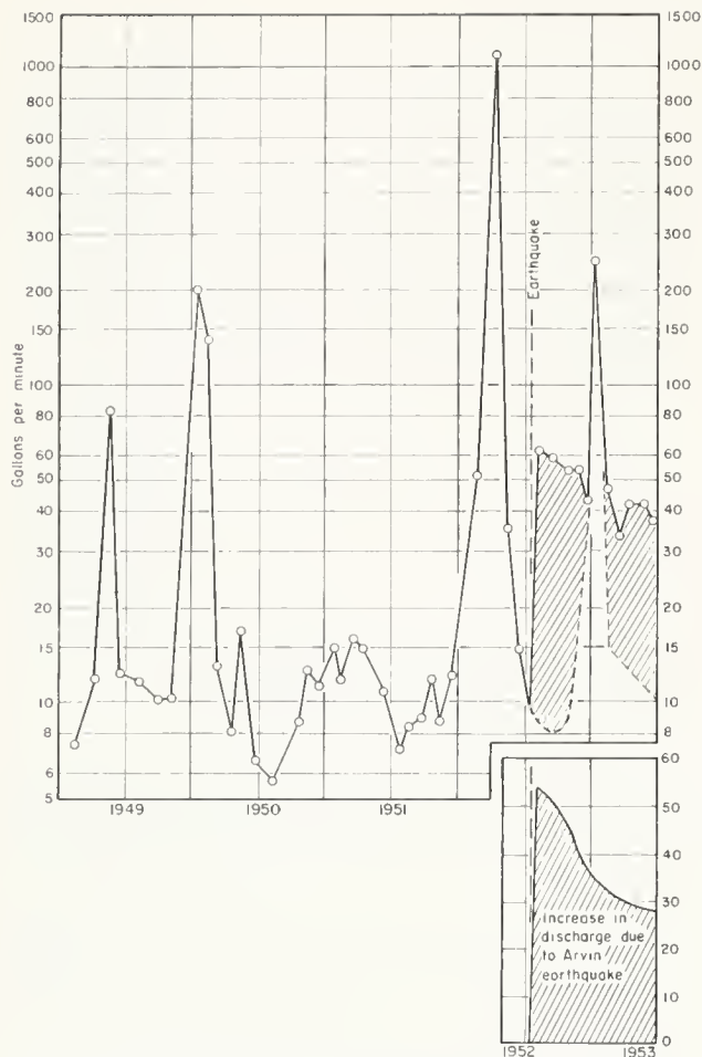
FIGURE 14. Hydrographs of discharge for San Jose Creek at Holme's place near San Marcos Pass.
