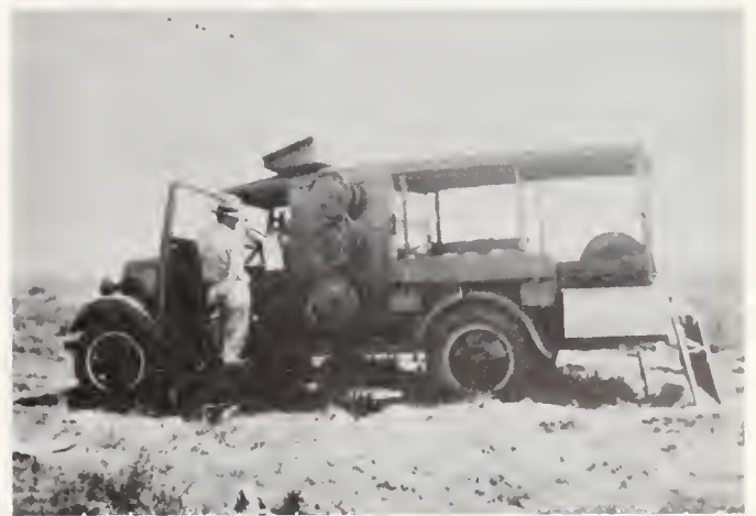
FIGURE 15. Early multitrace reflection seismograph recording truck used in the San Joaquin Valley, 1933. Courtesy Western Geophysical Company.
