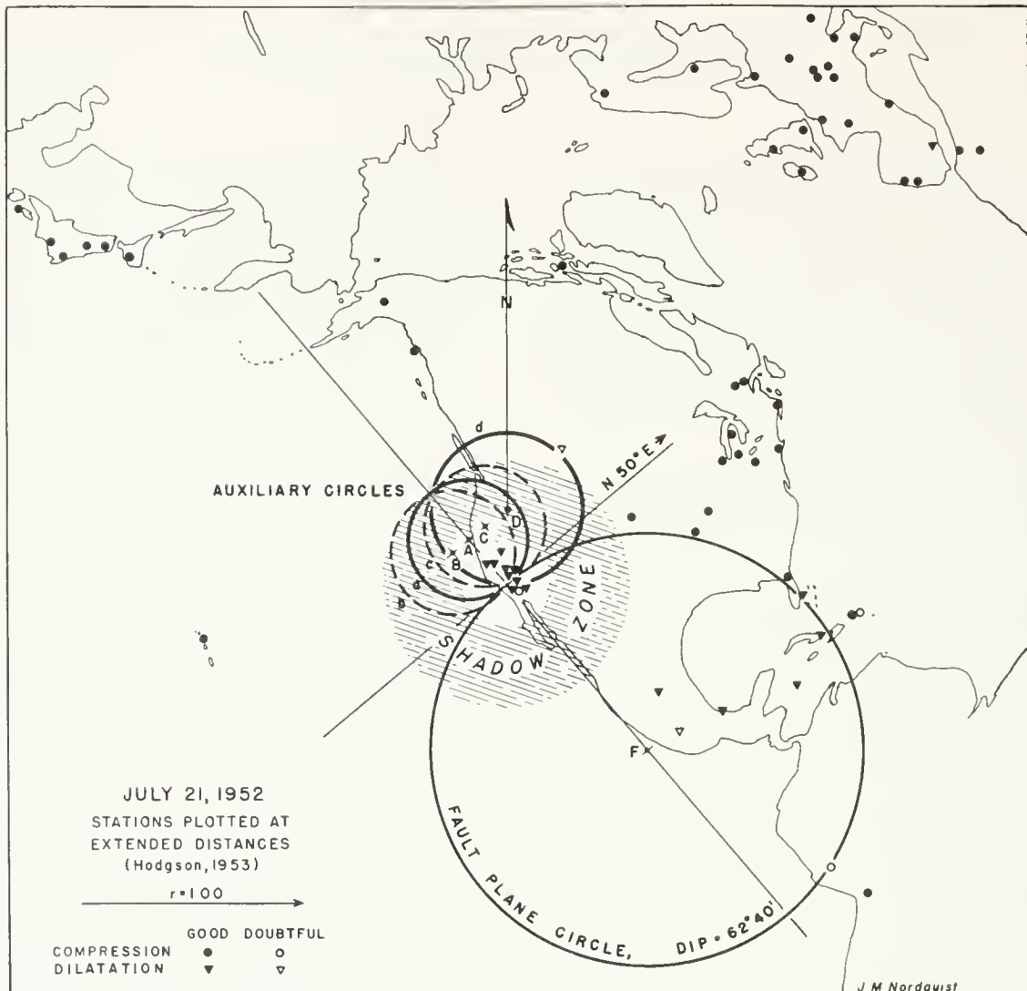
FIGURE 2. Observed compressions and dilatations in the main earthquake of July 21, 1952. For the projection, see text. The shadow zone for longitudinal waves is indicated by shading.
