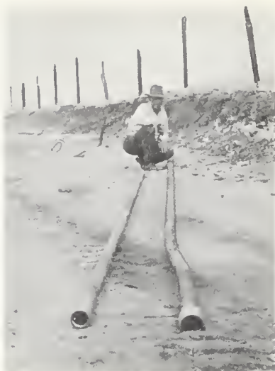
FIGURE 2. Twisted tubing pulled from a well where the casing had collapsed following the Arvin-Tehachapi earthquake of July 21, 1952.
