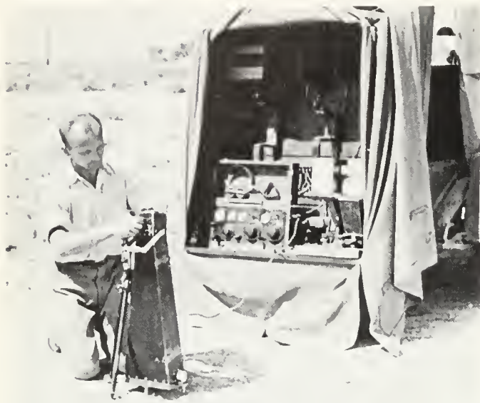
FIGURE 5. Adjusting mechanical seismograph, Shell Oil Company, 1928. Photo supplied by Frank E. Vaughan.
