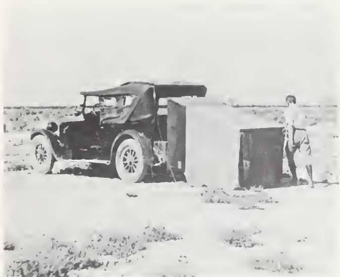
FIGURE 10. Recording car and tent enclosing seismograph, Shell Oil Company, 1928. Photo supplied by Frank E. Vaughan.
